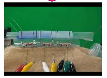
Movement of a actual esophagus is simulated using the function of shape memory alloys.
